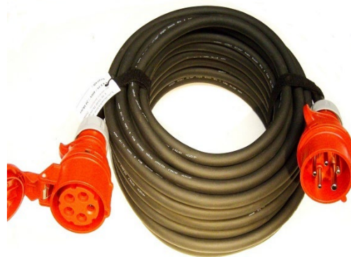
CEE16/5/400V/5x1.5mm2 oder 5x2.5mm2 Typ 66-1 = 5x1.5mm2 -8kW Typ 66-2 = 5x2.5mm2 -11kW
